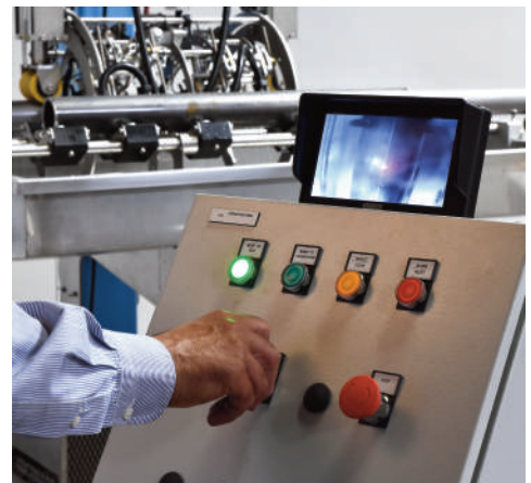
The remote operator station contains essential controls including the video monitor for checking transducer positioning with respect to the weld-zone, and the “joystick” for making adjustments.
