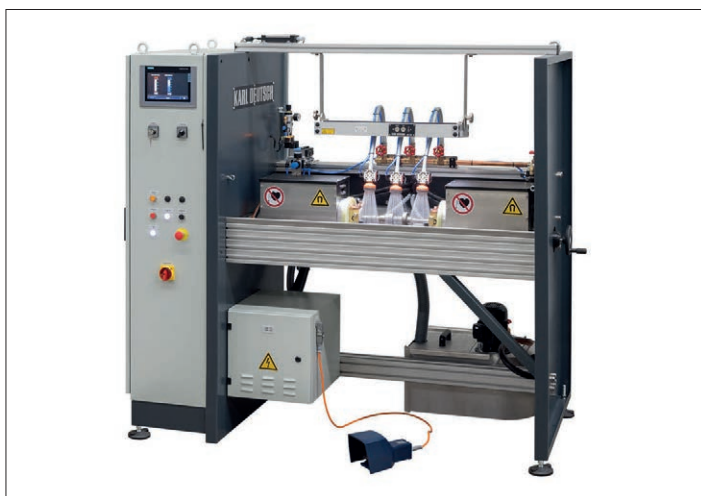
UWE 350: The image shows a unit equipped with Memory II and spraying showers (option).
