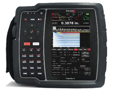
The instrument can be used with EMAT and piezoelectric sensors from Innerspec Technologies and other manufacturers. A setting of 600Vpp (approx. 3kW) is also available to maximize battery life if the application does not require full power.
