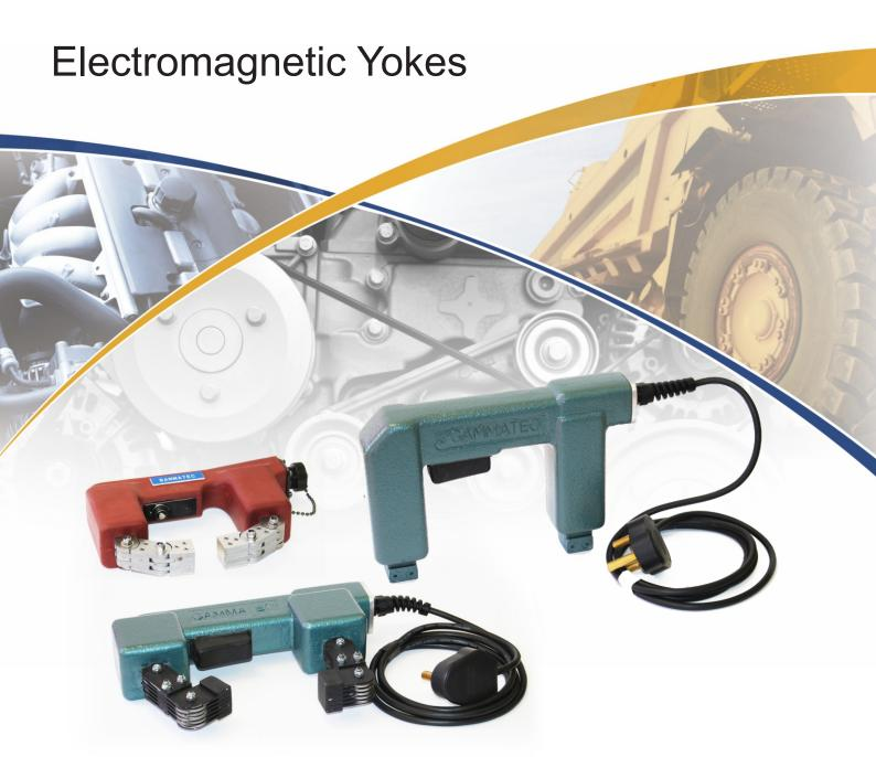
Gammatec's electromagnetic AC yokes are low cost, portable instruments which provide fast and accurate defect and crack detection in ferrous metals. The electromagnetic yokes are rugged and induce a powerful AC magnetic field. The adjustable poles and single handed operation makes our yokes ideal for inspecting components of different geometry – welds, castings and onsite inspection / repairs, especially where there is limited access.
